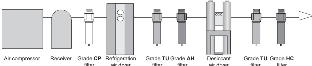
Note: 1. Grade TU filters after desiccant air dryer is for particle removal. Must be installed reversely and auto drain is unnecessary.
